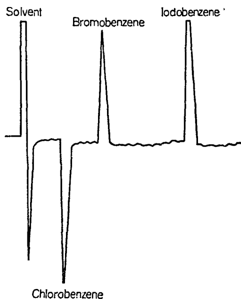
FIGURE 11. A typical chromatographic trace for a mixture of organic halides using the alkali flame detector of Figure 9. The sign of the bromobenzene peak can be inverted by narrowing the electrode gap (Figure 10) 397 . Reproduced by permission of Elsevier Publishing Co. from S. Lakota and W. A. Aue, J. of Chromatogr. , 44, 472 (1969).
